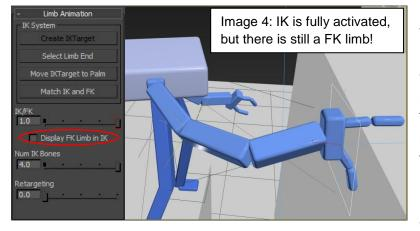
From the animation point of view, I was really appreciating the use of inverse kinematics controllers and link constraints. They make it easy to link parts of the rig to the environment or the other way around. A tricky part is probably to get an understanding for those two modes: When you're using inverse kinematics (IK), the forward kinematics 'version' (FK) of the limb can still move around and produce
